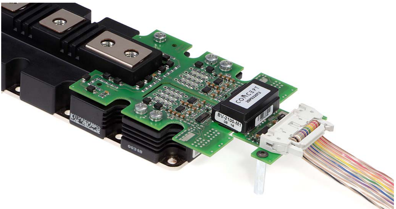
Fig. 11 Additional measures for fixing the driver
