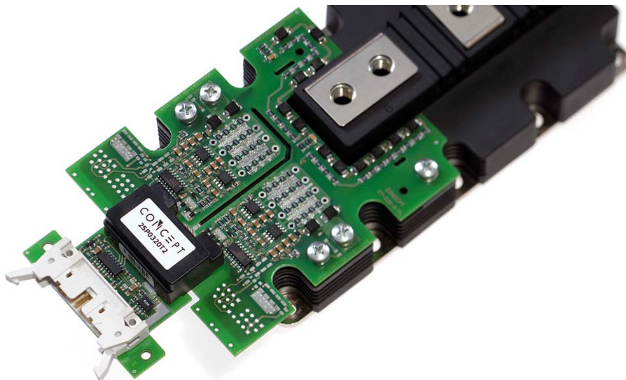
Fig. 1 2SP0320T screwed onto a PrimePACK™ IGBT module
