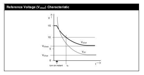
After  $t_{bl}$  has passed, the V<sub>CE</sub> monitoring will be triggered as soon as  $V_{CE} > V_{CEref}$  and will turn off the IGBT. The error memory will be set, and the output PRIM\_HOLD\_OUT changes to the HIGH state. Possible failure modes are shows in the following pictures.
